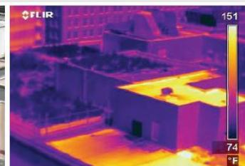
On a typical day, the Chicago City Hall green roof measures almost 80°F (40°C) cooler than the neighboring conventional roof.
